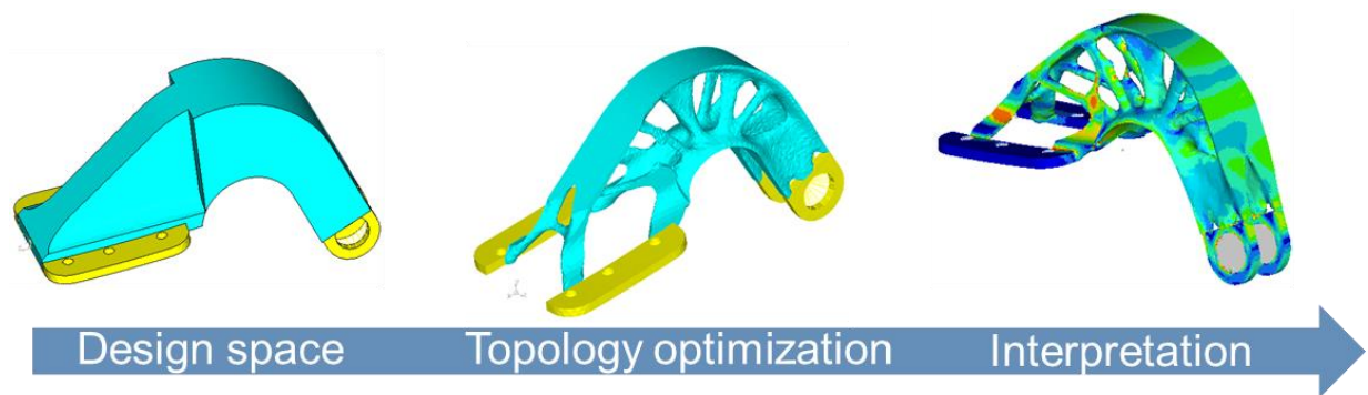
Figure 3.33 – Optimization of the Global APU door hinge from the design space to the interpretation
