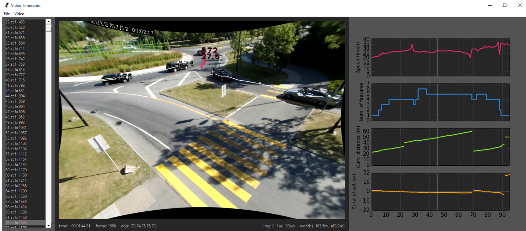
Figure 3.14 tvaLib GUI for trajectory, infraction, ground truth, and interaction playback.
