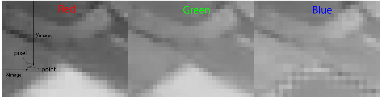
Figure 3.5 Close-up of image space for each of the three RGB channels. Note how the red and green channels have much more contrast than the blue channel. The bottom triangle is the end of a yellow crosswalk, the top triangle is a curb, and everything else is pavement.
