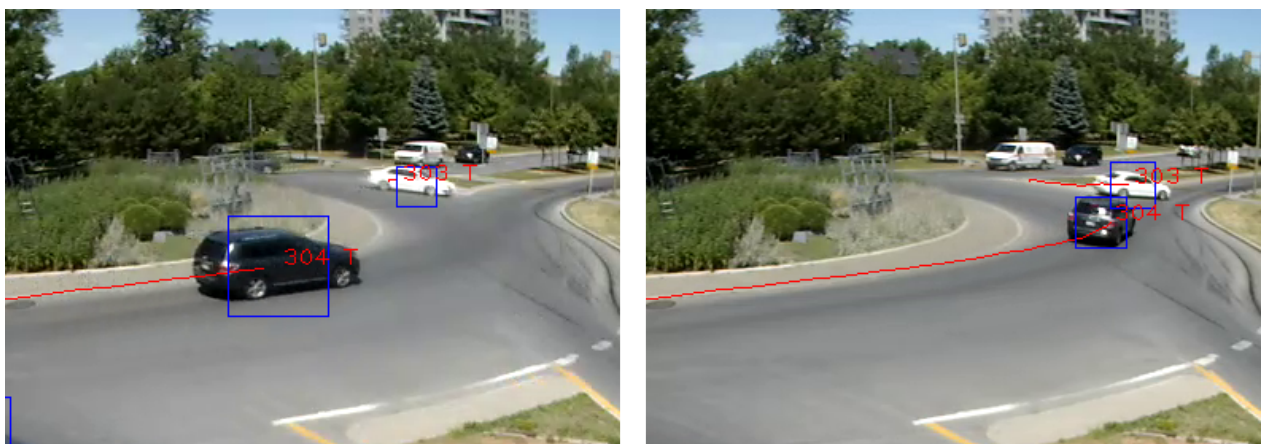
Figure 3.4 Example feature tracking (after feature grouping) of two vehicles in the scene.
