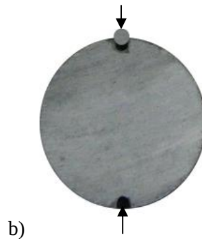
Figure 4-2: a) Roughness of the fracture obtained from different loading modes on Gabbro samples (Khosravi et al. 2014); b) Cylindrical sample with notches and round bar on the top.
