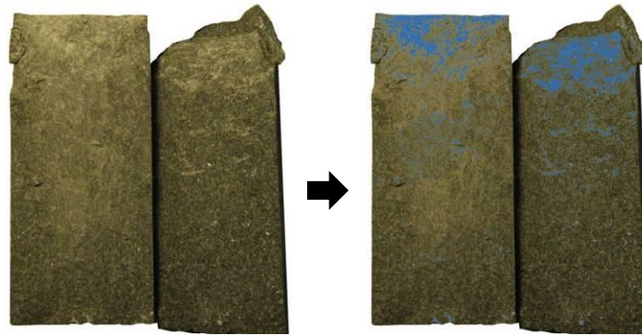
Figure 6-20: Contact area on the failure plane induced by a uniaxial compression test on basalt.
