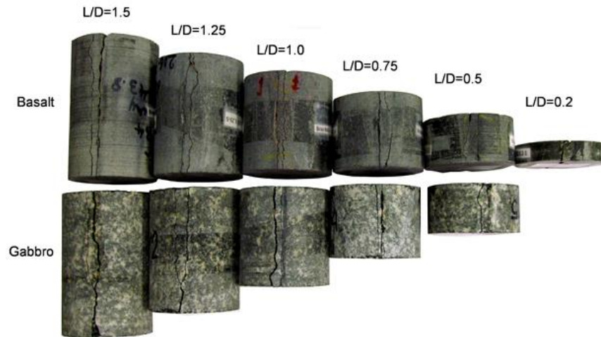
Figure 4-11: The size of wedge along the length of the specimens (gabbro and basalt).
