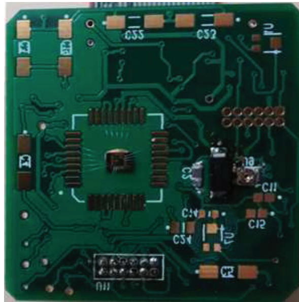
Figure 6.4 The power recovery unit assembled on a miniature PCB.
