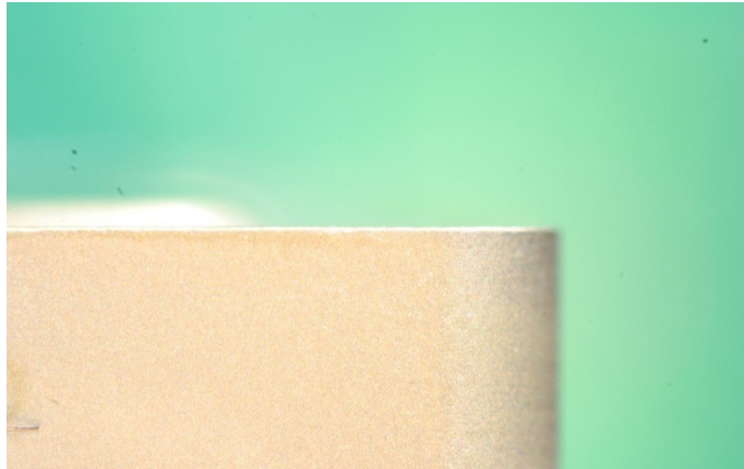
Figure 3-6 : Zero tool wear in a brand new insert
