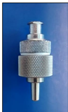
Filter holder 13 mm dia.
