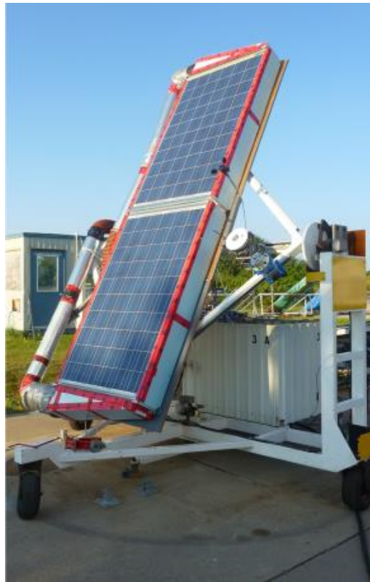
Figure 4-2: PV-T collector mounted on the outdoor combined PV and thermal testing rig
