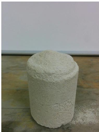
Figure 5.3 Échantillon post-rupture
