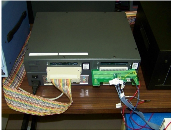
Fig. 4.5 The real time simulator (MX-station), the analog card (left), the digital cards (right)
