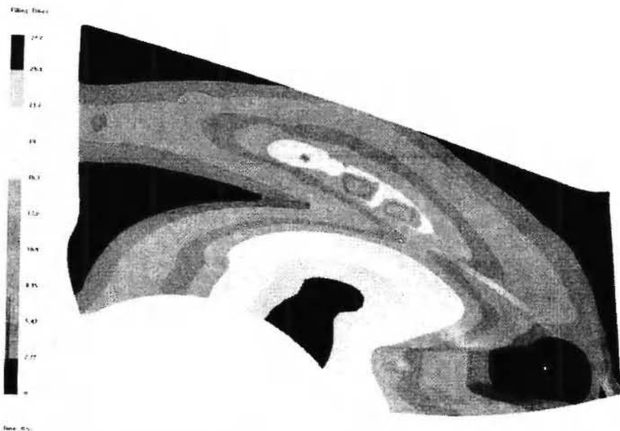
Fig. 26: Predicted flow front positions with the triangular mesh with the top foam skin permeability. A filling time of 27.2 sec was calculated.
