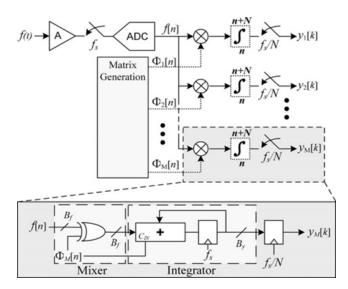
Figure 2.23 Block diagram of CS encoder [134]
