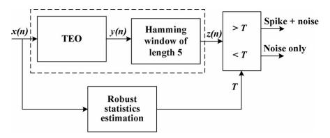
Figure 2.12 Block diagram of STEO-based spike detection with adaptive threshold [90]
