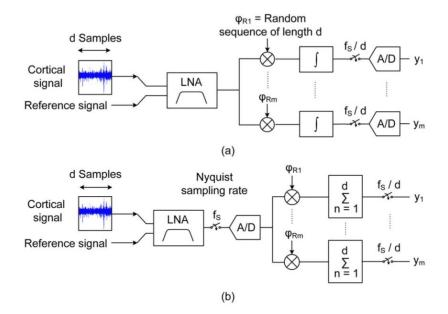
Figure 2.19 Block diagram of (a) the analog single-channel CS, (b) the digital single-channel CS
