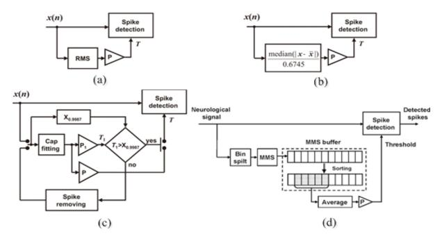
Figure 2.9 Comparison of four digital estimators, (a) RMS estimator, (b) MAD estimator, (c) Cap fitting estimator, (d) MMS estimator [96]
