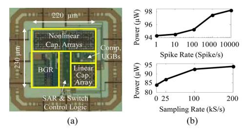
Figure 2.5 (a) Chip photograph of the proposed nonlinear ADC, (b) power consumption of the chip versus sampling rate (bottom) and spike rate at 200 kS/s (top) [42]
