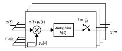
Figure 2.21 Block diagram of random demodulator pre-integrator (RMPI) [148]
