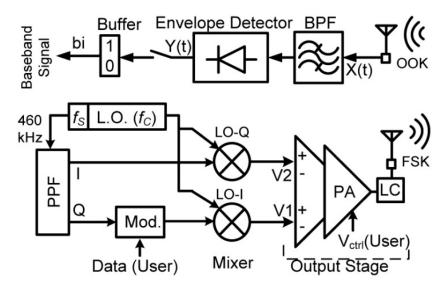
Figure 2.6 Block diagram of the proposed combined transceivers [45]
