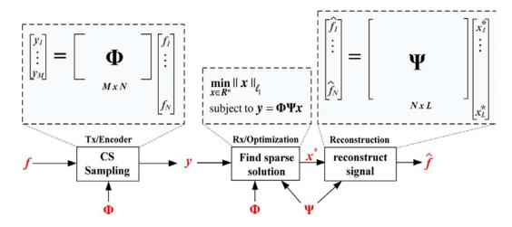
Figure 2.18 Diagram of CS sampling framework [134]
