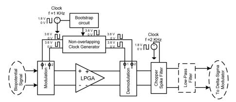
Figure 2.3 The chopped logarithmic programmable gain amplifier [36]
