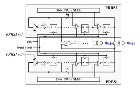
Figure 2.24 Block diagram of the measurement matrix generation block [134]
