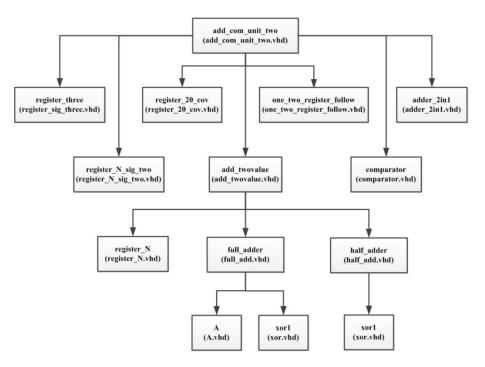
Figure C.8. The structure diagram of the add\_com\_unit\_two block
