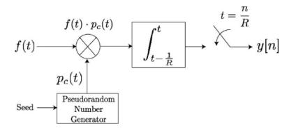
Figure 2.20 Block diagram of the random modulator [149]
