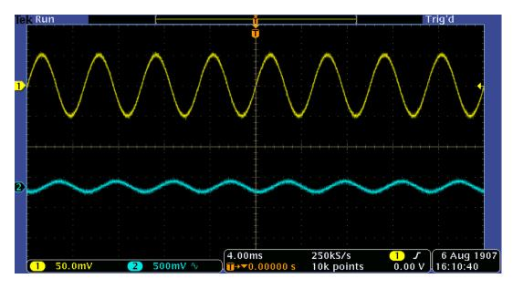
Figure B.3 Bandpass filter output is 300 mV (blue) for a 100 mV input (yellow) to the AD620 with the gain of 10. The input of the filter is 1Vpp. Frequency = 200 Hz
