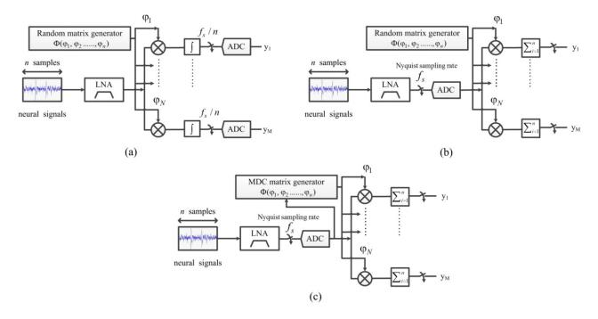
Figure 5.3 Diagram of the circuit design using the CS technique: (a) analog design, (b) digital design, (c) proposed digital circuit design using the MDC matrix
