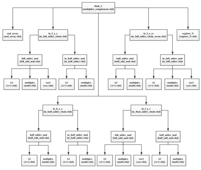
Figure C.9. The structure diagram of the Multi\_C block
