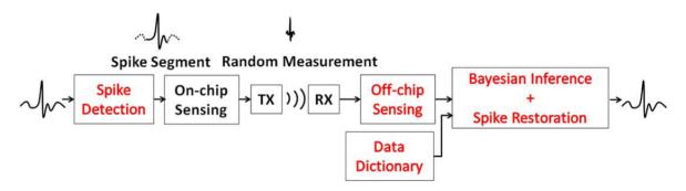
Figure 2.25 Proposed data dictionary based CS system [156]
