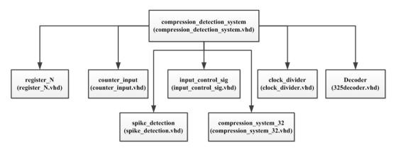
Figure C.2. The structure diagram of the compression\_detection\_system block
