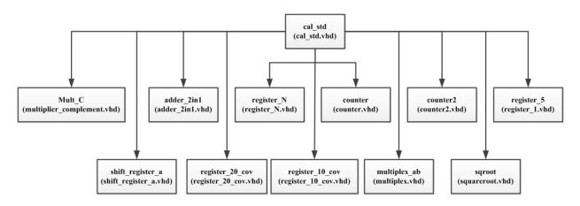
Figure C.5. The structure diagram of the standard deviation calculation block
