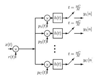
Figure 2.22 Block diagram of SRMPI [148]
