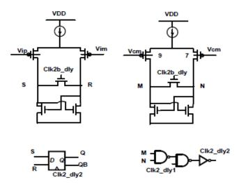
Figure 2.10 An analog self-timing static detector [101]
