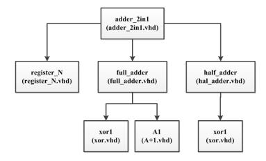
Figure C.10. The structure diagram of the adder\_2in1 block
