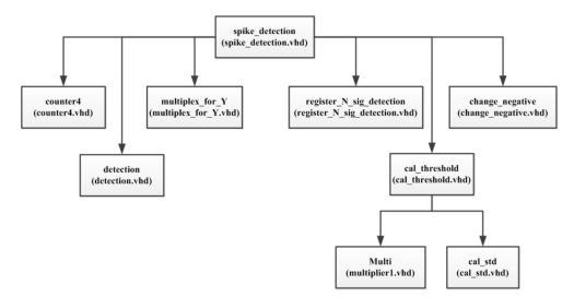
Figure C.3. The structure diagram of the spike\_detection block
