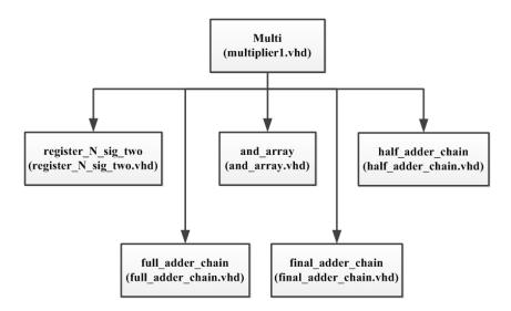
Figure C.4. The structure diagram of the multiplier1 block
