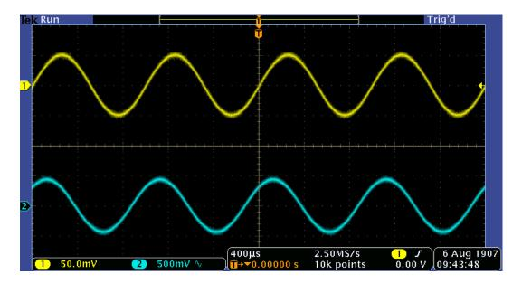
Figure B.5 Bandpass filter output is 1 V (blue) for a 100 mV input (yellow) to the AD620 with the gain of 10. The input of the filter is 1 Vpp. Frequency = 1 kHz
