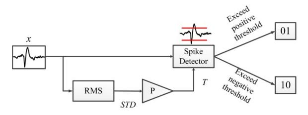
Figure 5.5 Diagram of the spike detection block
