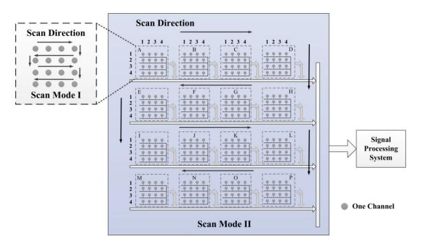
Figure 5.7 Diagram of the multichannel system
