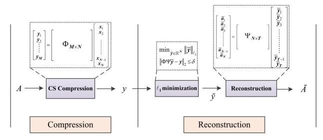
Figure 5.2 Framework of the compressed sensing technique
