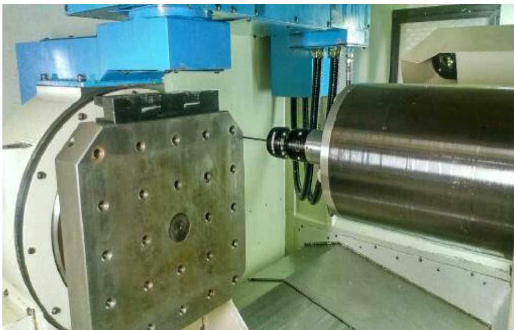
Figure 7-1 Probing on a WCBXFZYT machine tool
