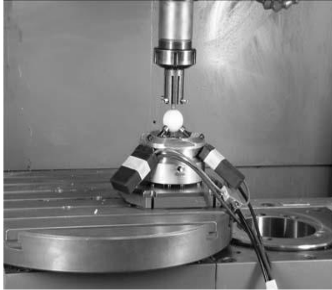
Figure 2-12 R-test device mounted on a five-axis machine tool (Weikert and Knapp 2004)
