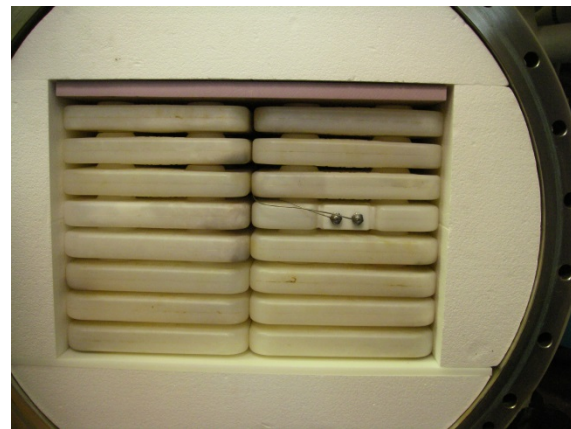
Figure 6-17: Insulated PCM storage tank
