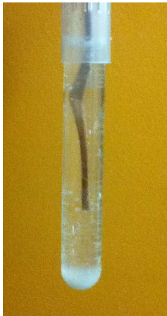
Figure A-1: Image of S27 sample equipped with a thermocouple sensor
