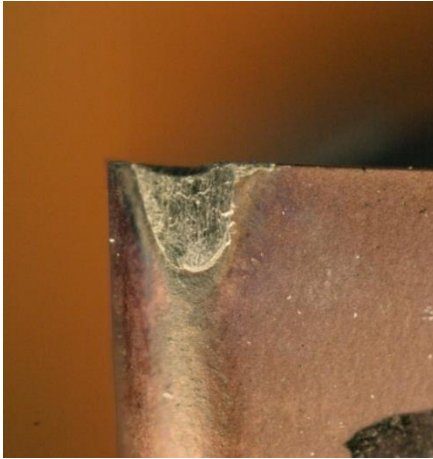
Figure 4-10: Carbide insert after turning Ti-MMC under following cutting conditions Cutting volume 9,000\text{mm}^3 , v_c=80\text{m/min} ; f_r=0.25\text{mm/rev} ; a_p=0.2\text{mm}
