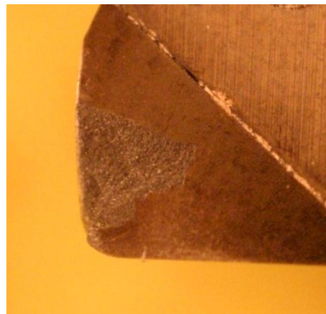
Figure 5-12: Wear in the PCD tool at v_c=450 \text{ m/min} , f_r=0.3 \text{ mm/rev} and a_p=0.1 \text{ mm}
