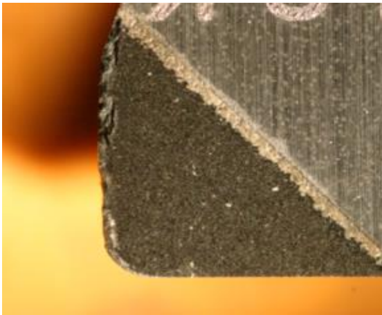
Figure 5-11: Edge chipping of the PCD at v_c=200 \text{ m/min} , f_r=0.17 \text{ mm/rev} and a_p=0.1 \text{ mm}
