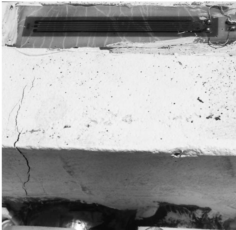
Figure 4.10 : Multi fine-crack around spliced - Specimen 35-F2-18D from IR2_F1 @ F_{max}
