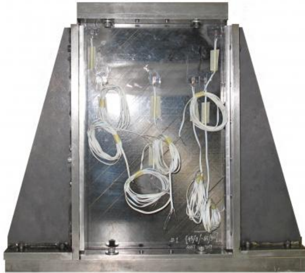
Figure 5.4 A test specimen mounted in the support fixture.
