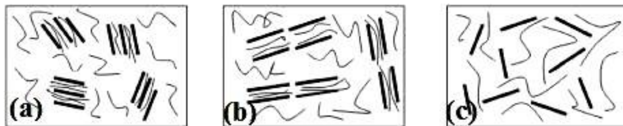
Figure 2.6: Schematic structure of three broad classes achievable polymer-clay nanocomposites; a) Intercalated, b) Intercalated and flocculated, c) Exfoliated structures [46].
