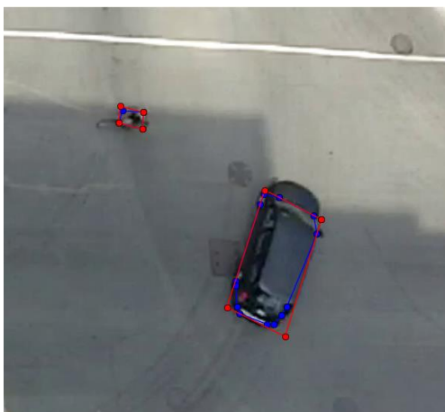
Figure 6.3: Examples of PET measurements (in the table under each image representing the interaction from the FBCH, FMAB, CirMB, CBM, and Manual methods)
