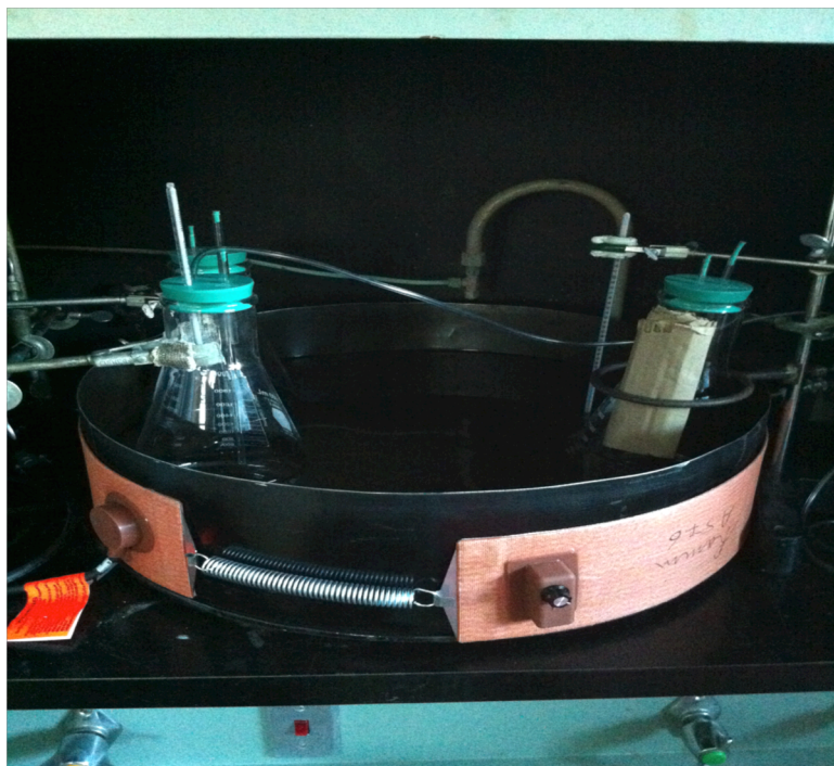
Figure 3.1-1 Composting bioreactors containing Sample, Positive control and Blank vessels.
