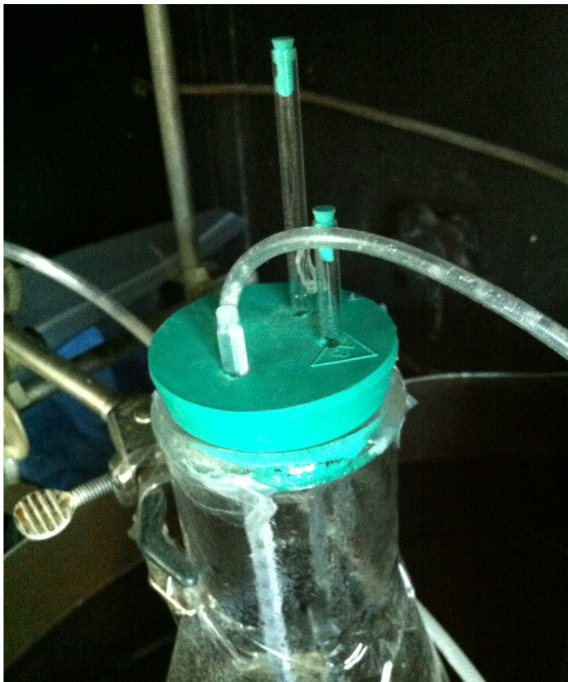
Figure 3.1-3 Composting vessel , two inlets for water and air and CO 2 outlet set at 55 °C
