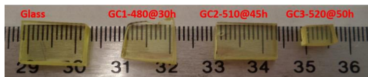
Figure 6-7: Photograph of the 2 mol. % Yb-doped glass and the glass-ceramic samples fabricated from a duplicate of the glass, after different annealing times.
