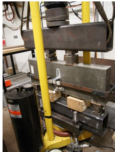
Figure 4.2 : Sustained loading test apparatus
