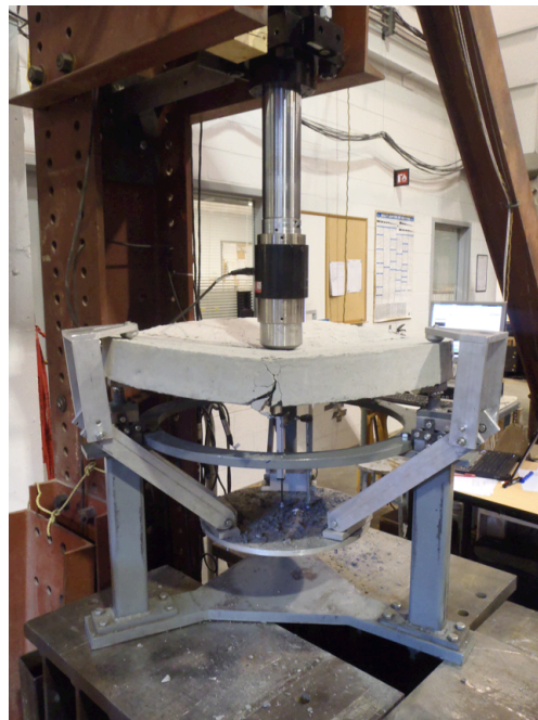
Figure A. 9: Apparatus used for the round panel tests at Polytechnique Montréal
