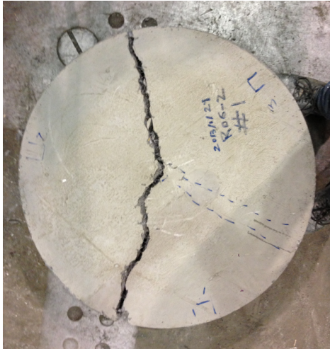
(a) Two-crack failure
