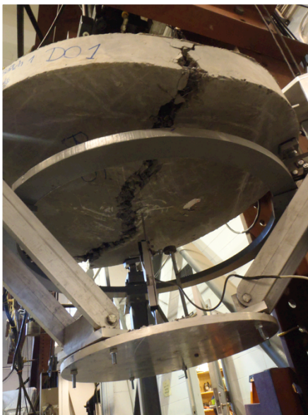
(a) failure with two cracks
