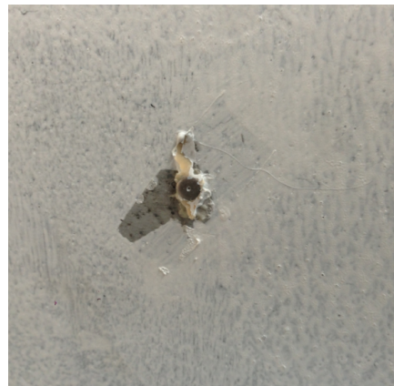
(b) Example of a DEMEC point
