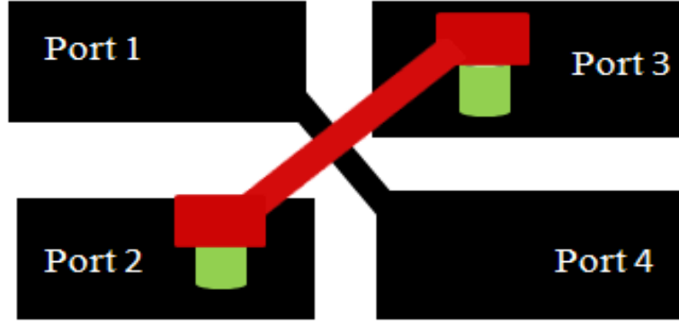
Figure. 5.23. Schematic representation of the ideal crossover junction, where ports 1 and 2 represent one transmission line and ports 3 and 4 represent the other transmission line.
