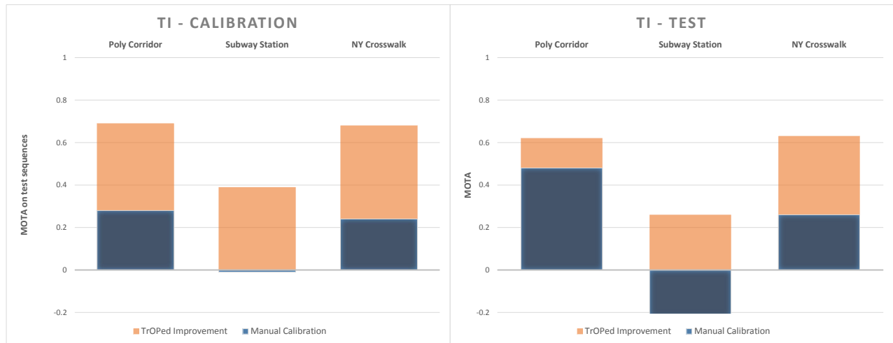
Figure 4.2 Comparison of manual and optimized parameter performance using Traffic Intelligence. Note that large negative values are not fully displayed.
