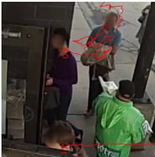
Figure 4.12 Example of Traffic Intelligence failing to dissociate visually distinct targets.
