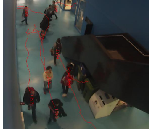
Figure 4.11 Example frame of Traffic Intelligence tracking on the Polytechnique calibration sequence.
