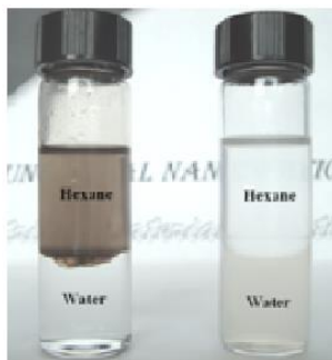
Figure 4-2: Optical photographs of \text{Fe}_3\text{O}_4@\text{OA} NPs, which can be easily dispersed in hexane (left); after silica coating, the \text{Fe}_3\text{O}_4@\text{SiO}_2 NPs can be dispersed in aqueous solution (right).
