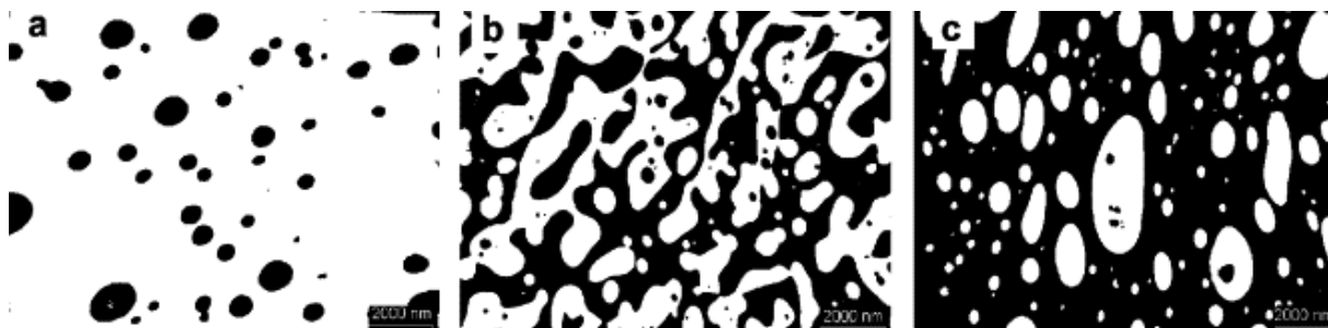
Figure 2.23: Transmission electron micrographs for PMMA/PS blends at different blend compositions: (a) 90/10, (b) 50/50, (c) 30/70 (Steinmann et al., 2001)
