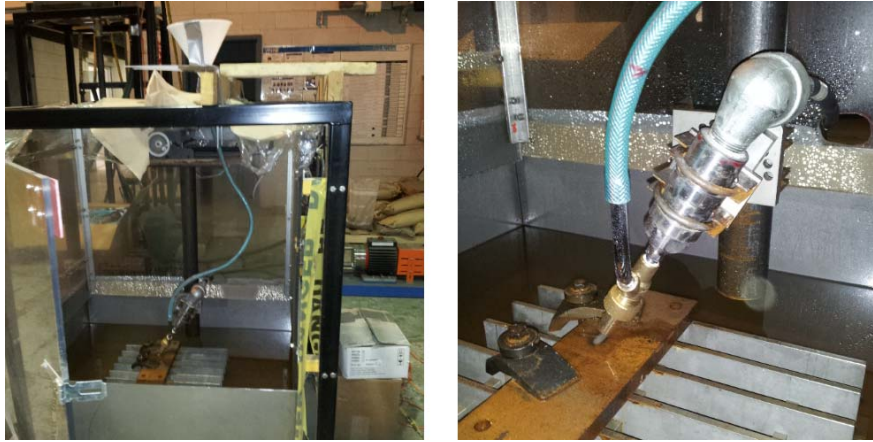
Figure 8.7 Abrasive feeding system used to add the abrasives to the jet inside the ejector in the modified test rig.
