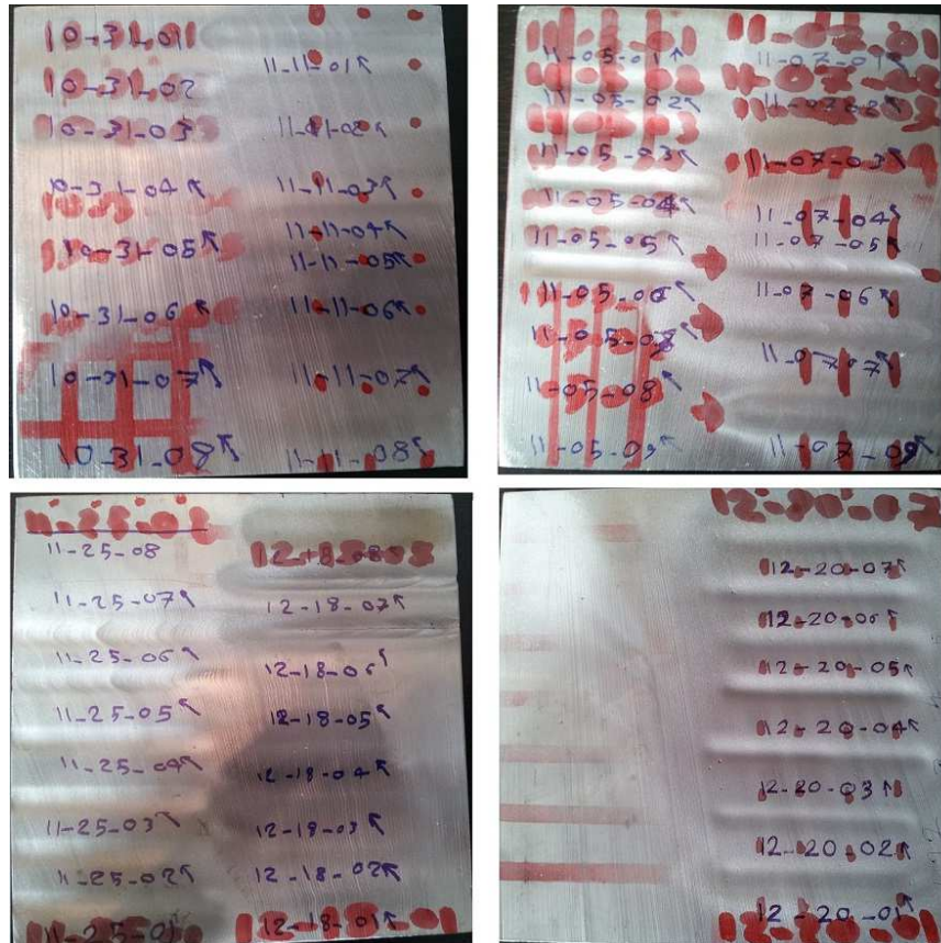
Figure 8.12 Polished lines on the workpieces obtained as the preliminary results of experiments on the AWJP process
