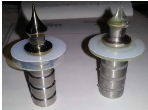
Figure 8.6 Comparing the worn plunger of the pressure valve (right) with the new one (left).
