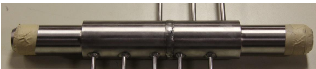
Figure 2.15 Photo of the test section showing the welded region.
