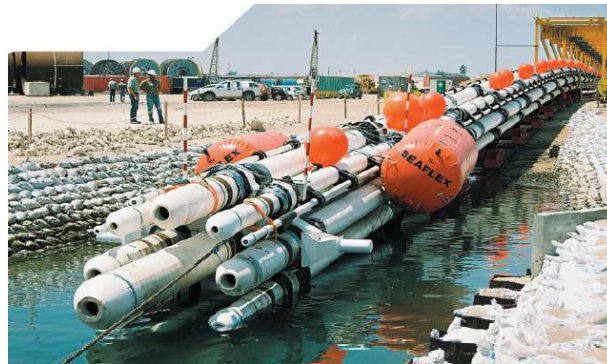
Figure 3.1 Riser tower bundle [9]
