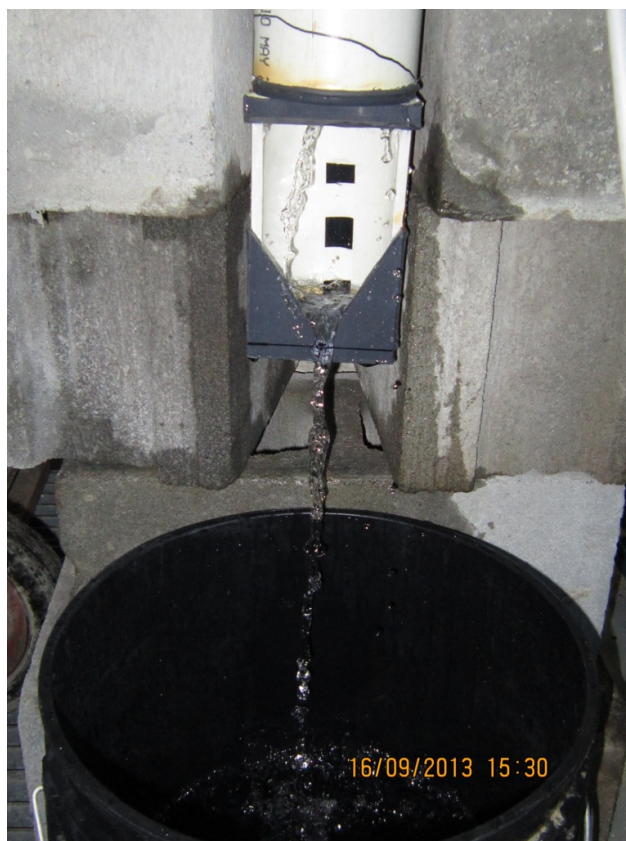
Figure 5.5 Front view of DFM calibration with graduated bucket.
