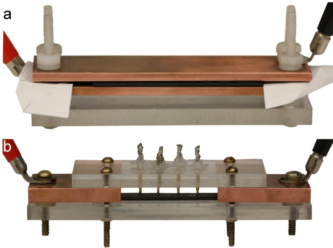
Figure 3-2 : (a) Sample holder used for electrical characterization of i) nanocomposite samples in directions parallel and perpendicular to the electric field, and ii) multiscale composite samples in the direction parallel to the electric field, i.e. through-the-thickness (TTT) of the sample; (b) Sample holder used for the electrical characterization of multiscale composite samples in the longitudinal direction, i.e. along the length of the samples (parallel to the carbon fibers)
