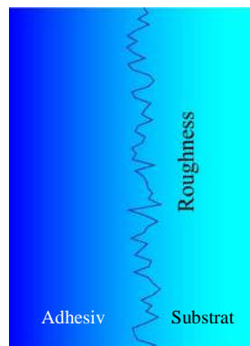
Figure 2-5: Schematic image of mechanical interlocking between adhesive and substrate due to solid rough surface.
