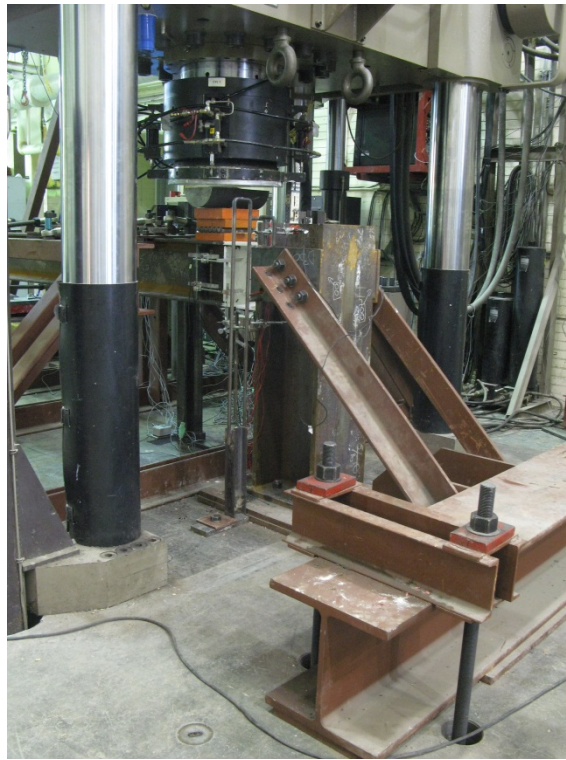
Figure 3-2 - Stub column, restraining vertical braces and floor beam
