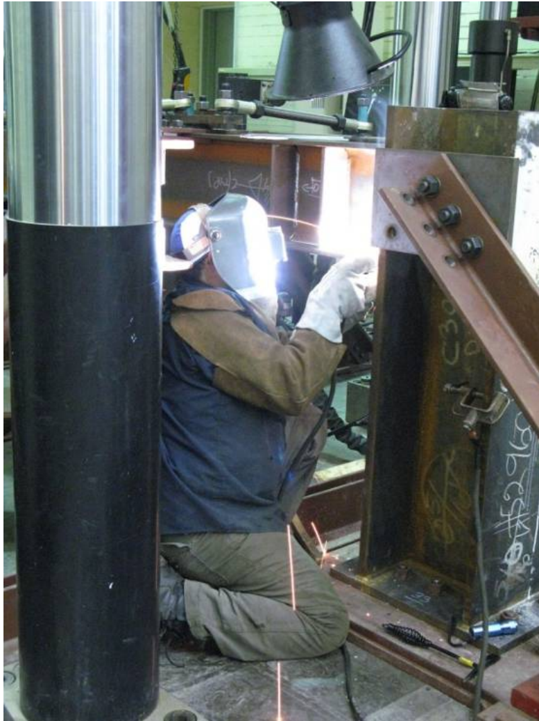
Figure 3-10 - Retrofit Weld Performed by Certified Welder
