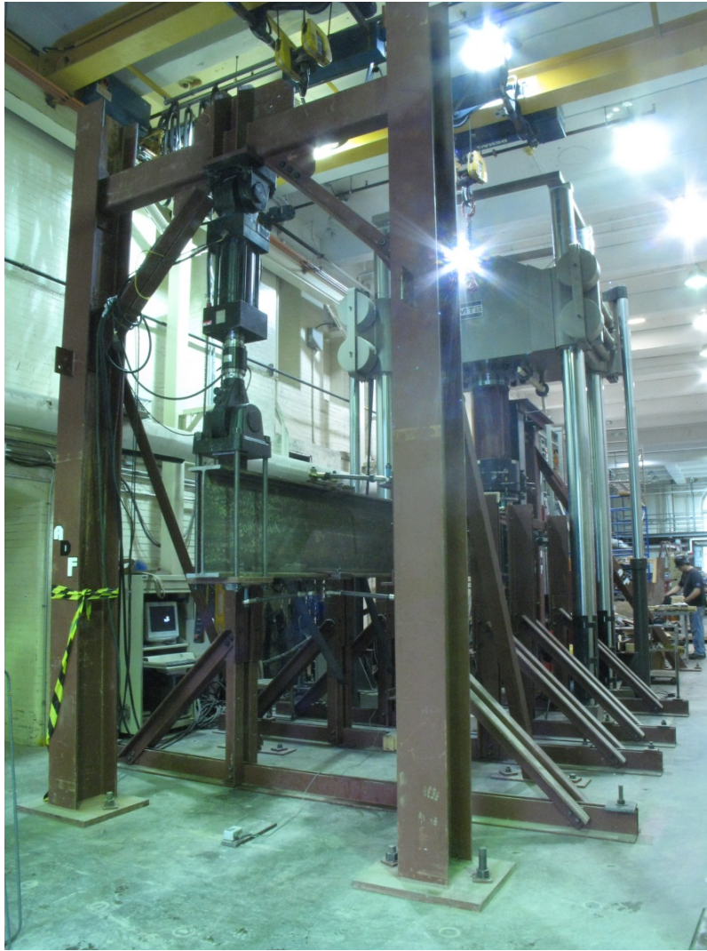
Figure 3-5 - End Frame and End Actuator for Flexible Support Setup
