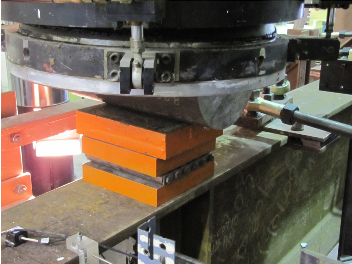
Figure 3-12 - Roller Set and Half Round Rocker
