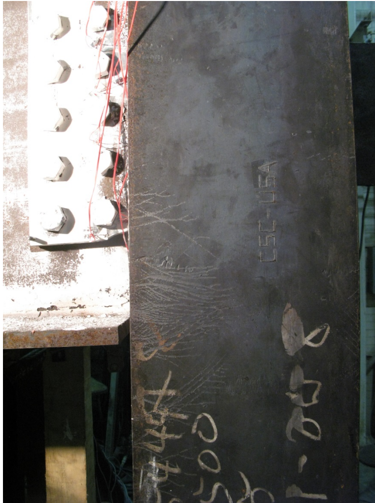
Figure 4-10 - Test 6 Column Showing Signs of Yielding
