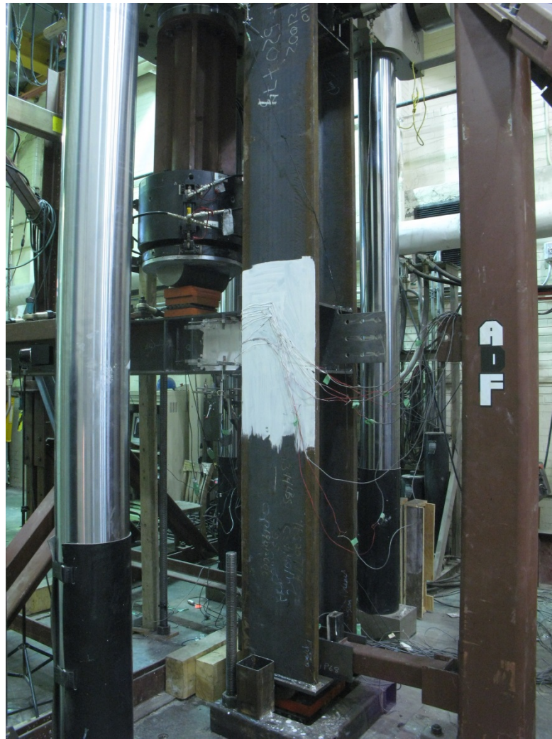
Figure 3-6 - Test Column End Restraints
