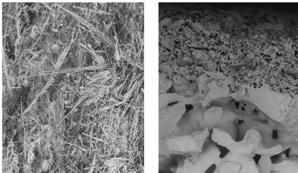
Figure 1-2 The structure of a low density (left) and high density (right) of porous ceramics[10]
