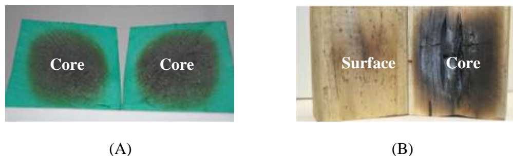
Figure 1-8: Materials heated by MWH, (A) rubber stopper and (B) wood cube
