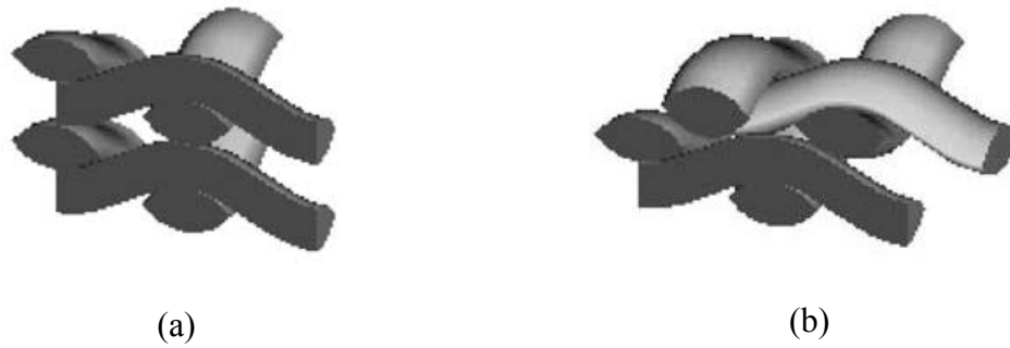
Figure 5-4: Extreme nesting cases: (a) no nesting and (b) maximum nesting (Lomov et al., 2003).
