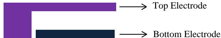
Figure 3-1: Structure of Capacitive sensor
