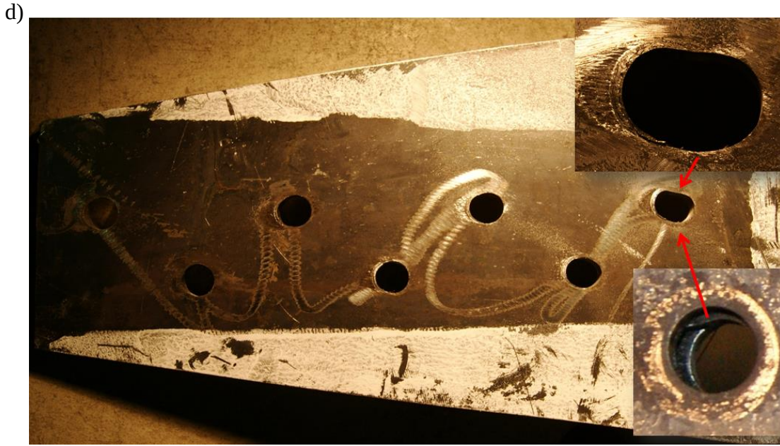
Figure 3.18: Specimen No. 1 - Damage to end connections after the test: a) yielding in the bottom connection; b) yielding in the top connection; c) residual deformed shape of the brace; d) hole elongation in the gusset plate (continued)
