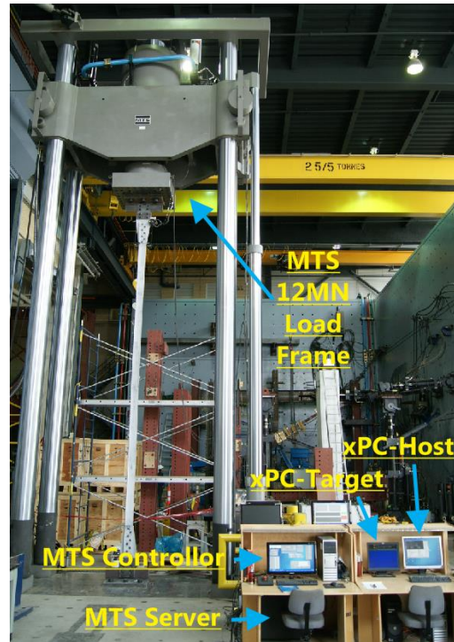
Figure 5.8: Photo of hybrid simulation setup
