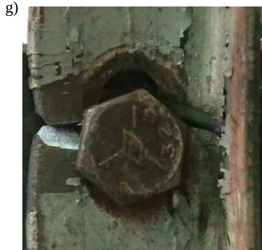
Figure 3.46: Specimen No. 5 - Net section of the old angle brace: a) before test; b) at initiation of yielding; c) upon increasing yielding; d) at necking; e) at initiation of cracking; f) at fracture of the critical region; g) near complete net section rupture (continued)
