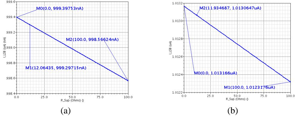
Figure 4.11:  $I_{LSB}$  reduction due to resistance of  $V_{dd}$  path (a) ideal bias; (b) designed bias;
