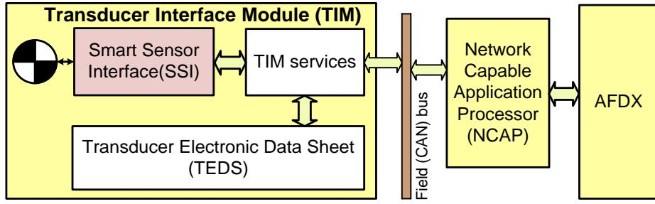
Figure 1.3: Architecture of modified AFDX network along with the SSI
