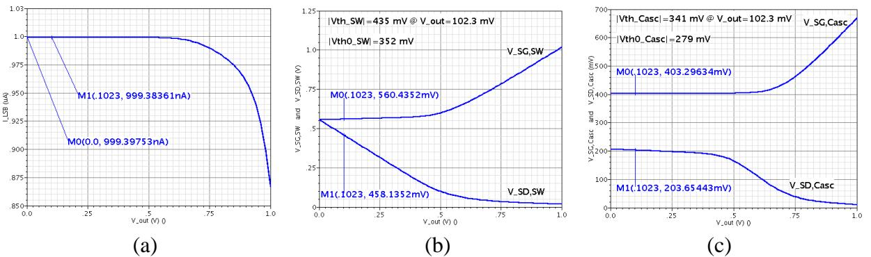
Figure 4.7:  $V_{out}$  effects (ideal bias) (a)  $I_{LSB}$ ; (b)  $V_{SG}$  and  $V_{SD}$  of  $M_{SW}$ ; (c)  $V_{SG}$  and  $V_{SD}$  of  $M_{Casc}$ ;
