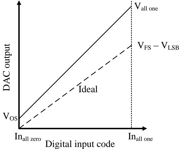
Figure 4.2: Offset and gain errors in CSDAC
