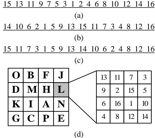
Figure 3.12: Switching sequences for a  $16 \times 16$  CSA; (a) Symmetrical sequence (b) Hierarchical-symmetrical sequence (Type A) (c) Hierarchical-symmetrical sequence (Type B) (d)  $Q^2$  random walk sequence [58]
