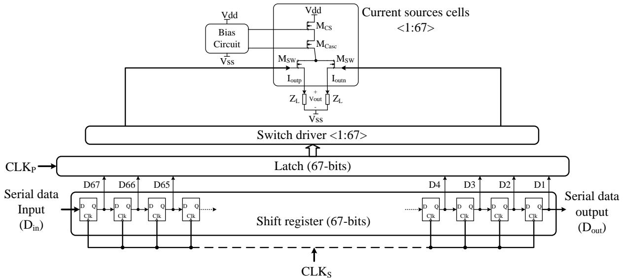
Figure 4.30: Functional block diagram of the designed SCSDAC
