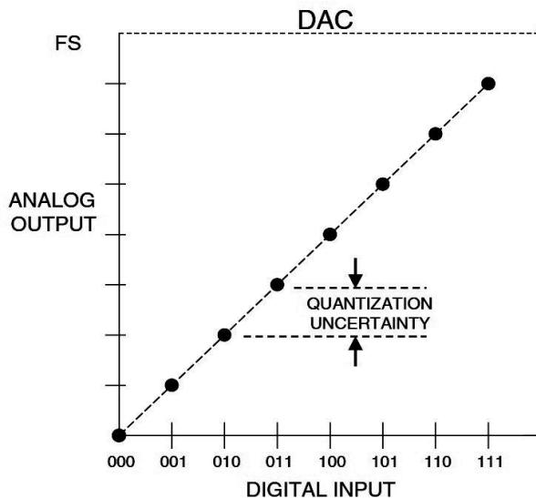
Figure 3.3: Transfer function of an ideal 3-bits DAC [49]
