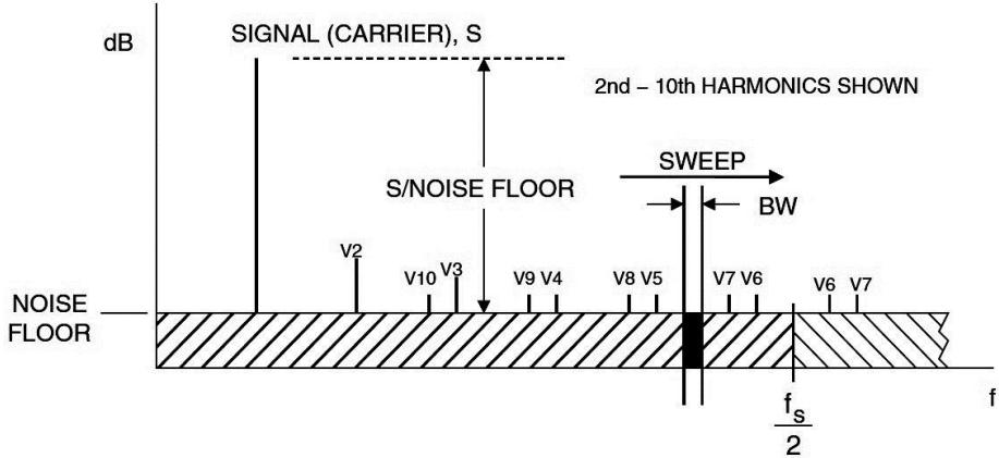
Figure 4.4: Frequency spectrum of DAC output [49]
