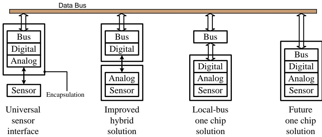
Figure 2.1: Several types of integrated sensing systems
