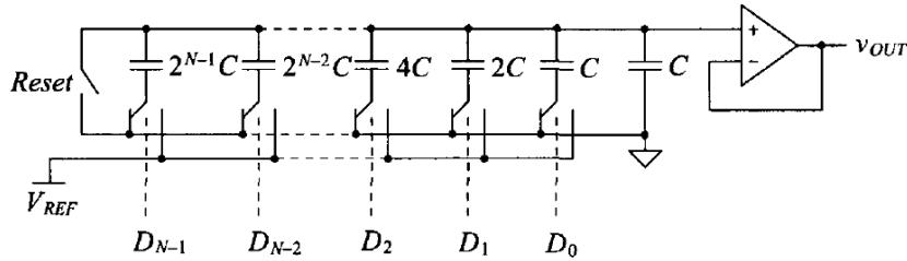
Figure 2.6: Binary-weighted charge-scaling DAC architecture [47]
