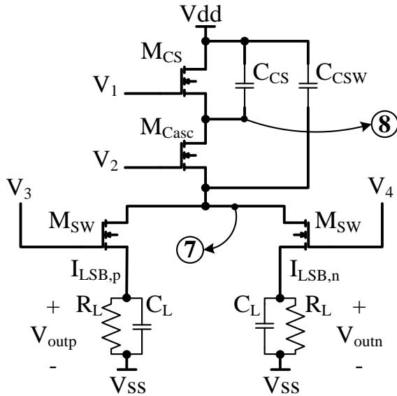
Figure 4.17: Equivalent circuit of LSB current source
