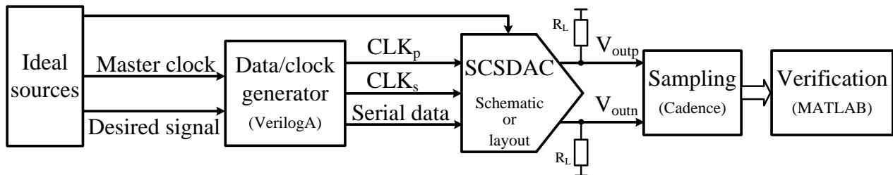
Figure 4.5: Test bench setup for DAC simulation
