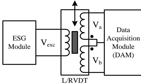
Figure 2.2: L/RVDT interface modules
