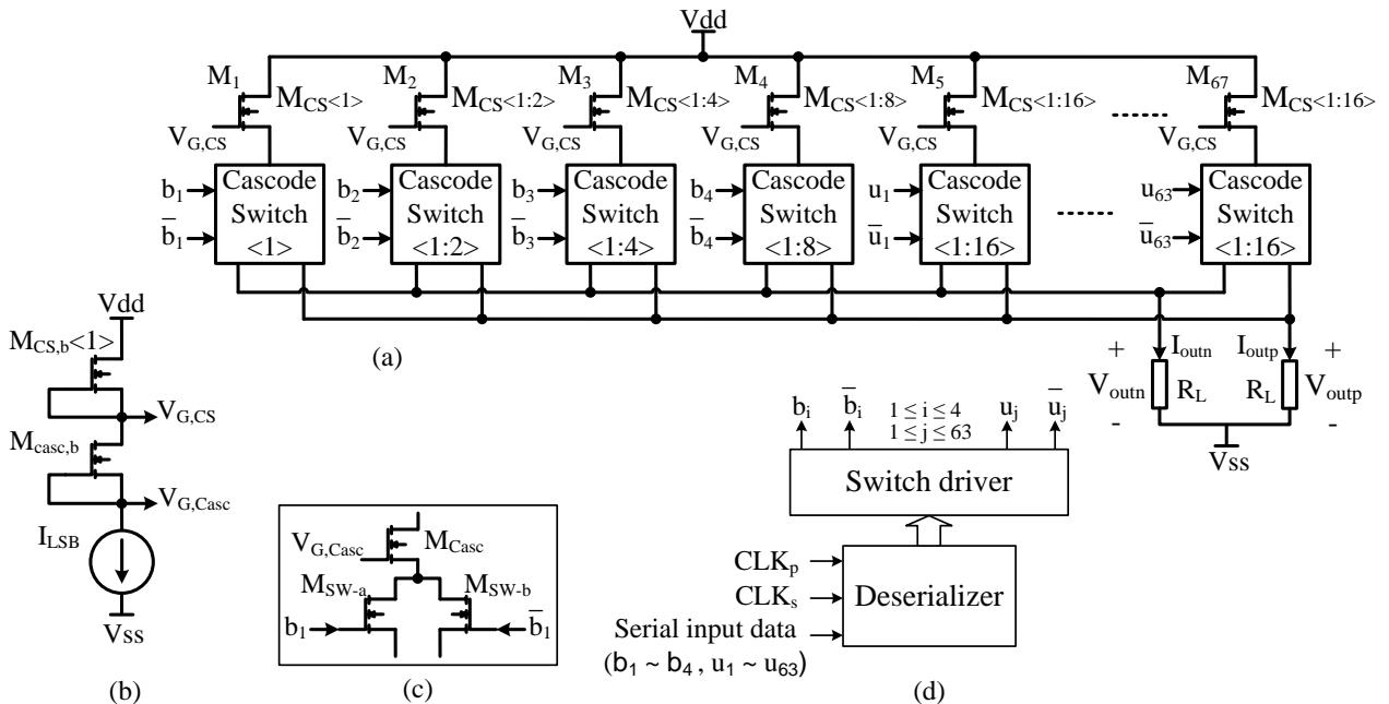
Figure 3.15: Detailed diagram of the proposed SCSDAC;
