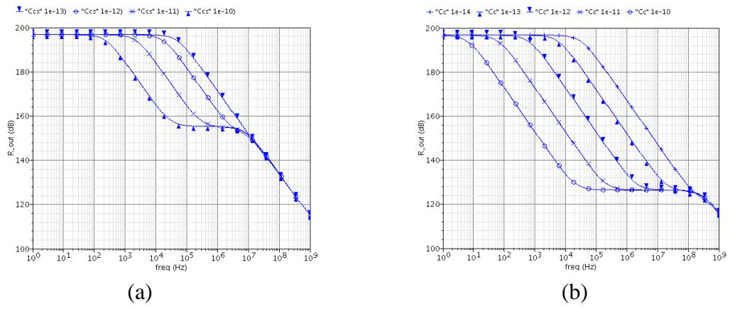
Figure 4.19:  $R_{out}$  of LSB source for various (a)  $C_{CS}$ ; (b)  $C_{CSW}$
