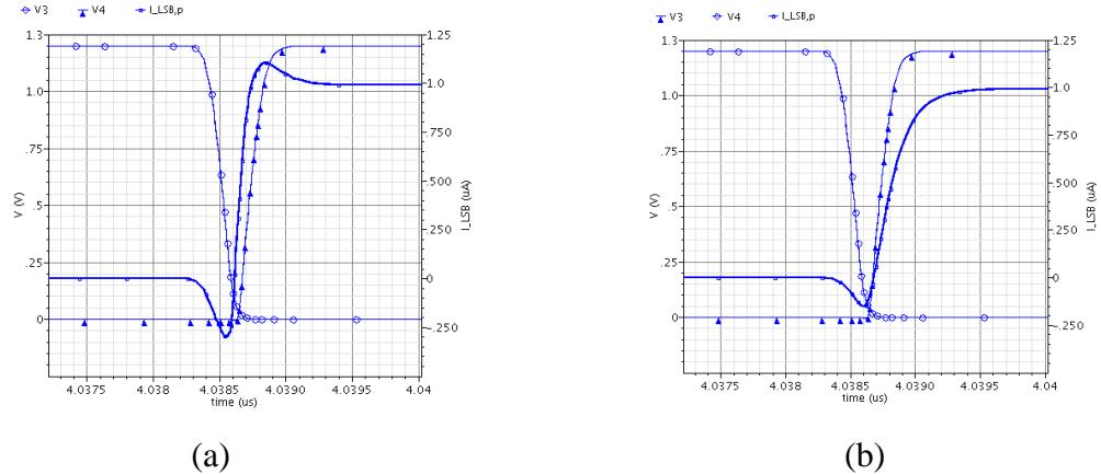
Figure 4.25: Effect of designed switch driver circuit on output step of  $I_{LSB}$ ; (a)  $C_L=0$  ; (b)  $C_L=2$  pF;
