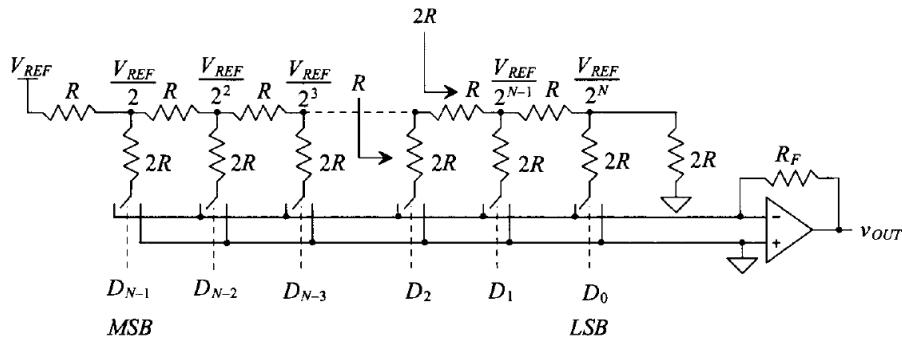
Figure 2.5: R-2R ladder DAC architecture [47]
