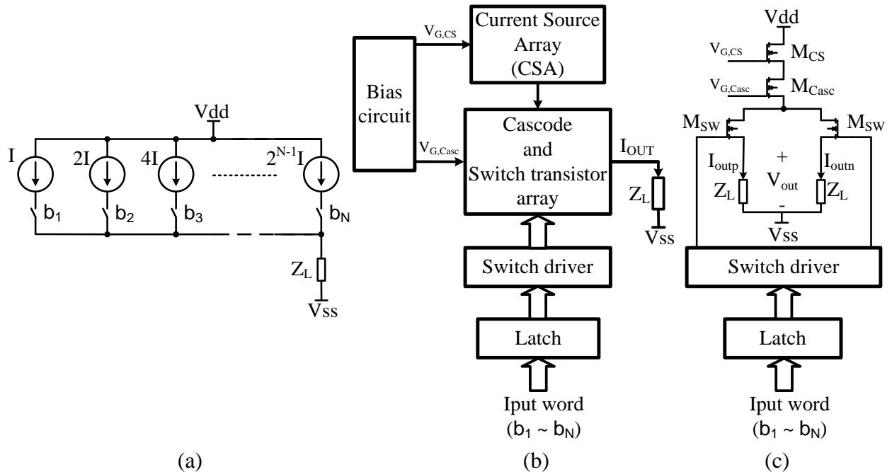
Figure 3.6: Binary-weighted CSDAC; (a) Conceptual diagram, (b) General block diagram, (c) Circuit diagram
