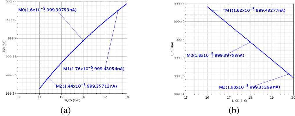
Figure 4.13:  $I_{LSB}$  aberrations due to size of  $M_{CS}$  with ideal bias circuit (a)  $W_{CS}$ ; (b)  $L_{CS}$ ;
