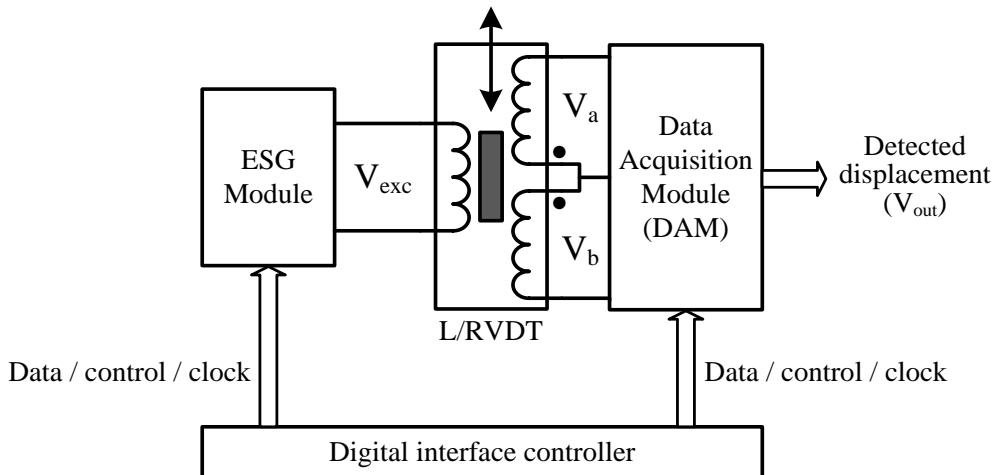
Figure 3.1: System level diagram of the SSI [1]
