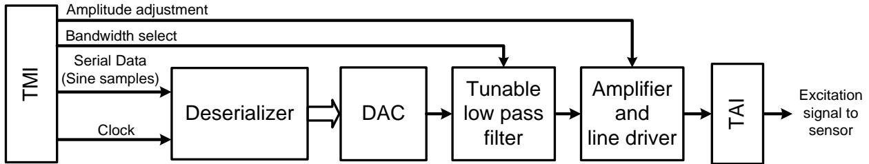
Figure 3.2: Proposed ESG architecture
