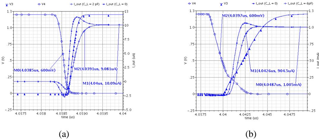
Figure 4.26: Effect of designed switch driver circuit on output step of (a) 10 $\mu$ A; (b)  $I_{FS}$ ;
