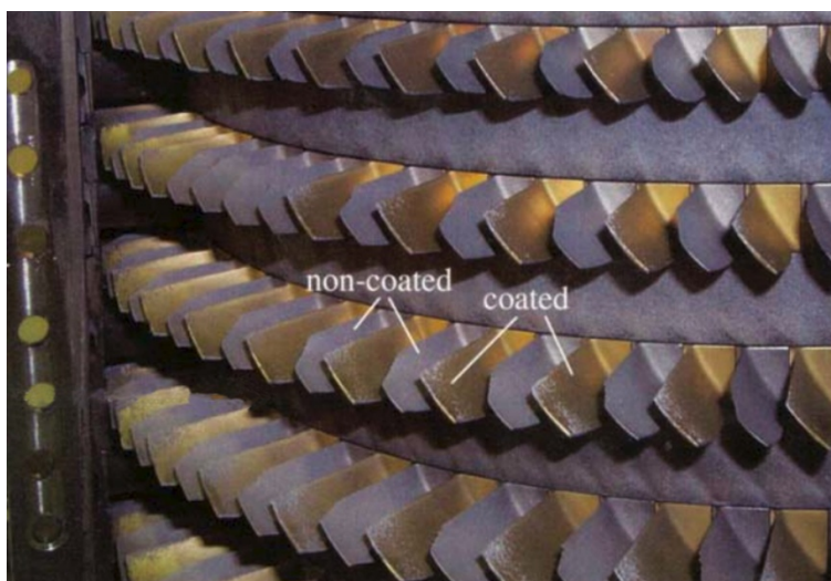
Figure 1.3: GE T64 jet engine compressor with half the blades coated with a TiN-based multilayer coating [7].
