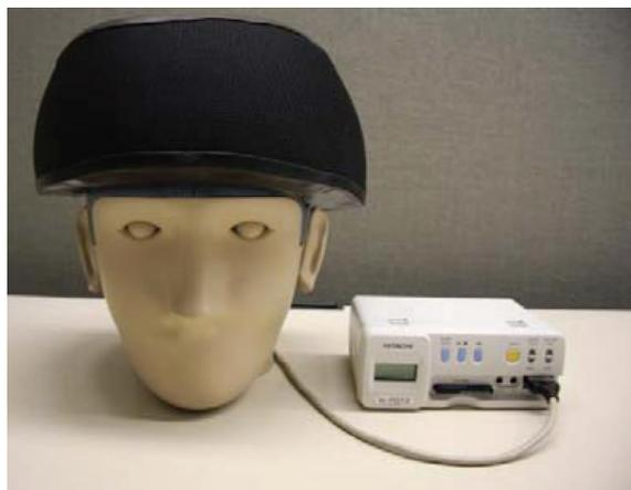
Figure 2.3: Prototype SPIR portable issu de Kiguchi *et al.* (2012))
