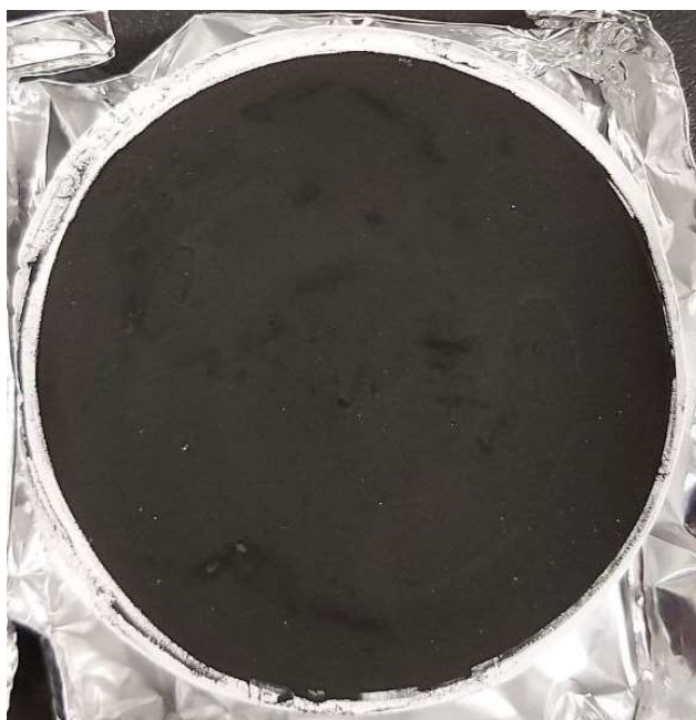
Figure 4-3 PAC accumulation on the filter surface after drying
