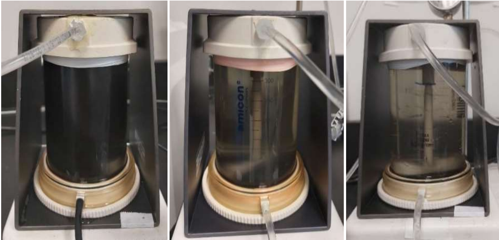
Figure 5-7 Amicon cell after treating 50, 100, and 125 L water/ g PAC respectively.
