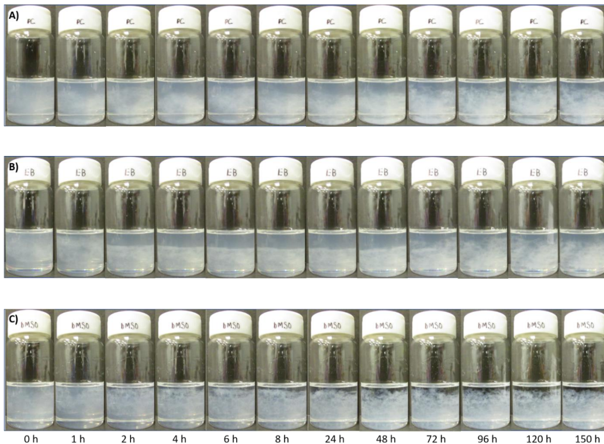
Figure B.3 Evolution of the dispersion state over time in A) propylene carbonate, B) ethyl benzoate and C) DMSO. Pictures of the vials were taken at 0, 1, 2, 4, 6, 8, 24, 48, 72, 96, 120 and 150 h after sonication.
