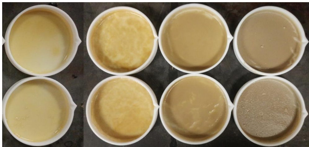
Figure 6.3 SBR composites obtained by solvent casting containing 0 wt% (a), 1 wt% (b), 5 wt% (c), and 10 wt% (d) of BNNTs.
