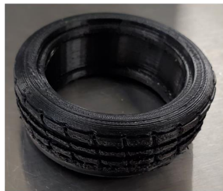
Composite F3, dimensions: 68.4 mm dia. x 27.0 mm H
