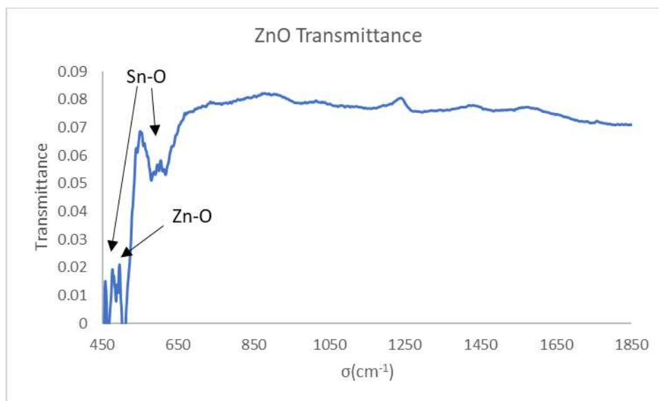
Figure 6.8: FTIR Spectrum of the transmittance energy variation with the wavelength for the ZnO layer deposited on FTO
