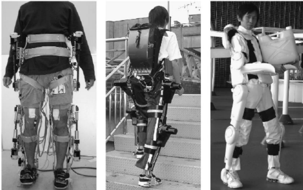
Figure 2.11 Evolution of the Hybrid Assistive Limb: HAL-1, HAL-3, and HAL-5 [56]
