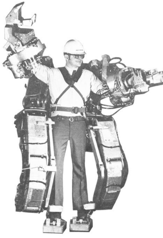
Figure 2.10 The Hardiman exoskeleton prototype, developed by General Electric [54].
