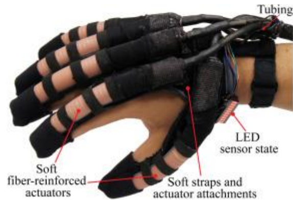
Figure 2.13 An example of soft actuators used for a hand exoskeleton prototype for assistance [79].
