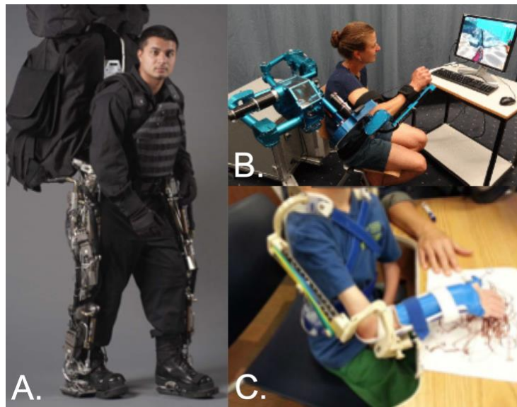
Figure 2.12 Example of an exoskeleton for A. Augmentation (BLEEX [57]), B. Rehabilitation (ChARMin [58]), and C. Assistance (WREX [59])
