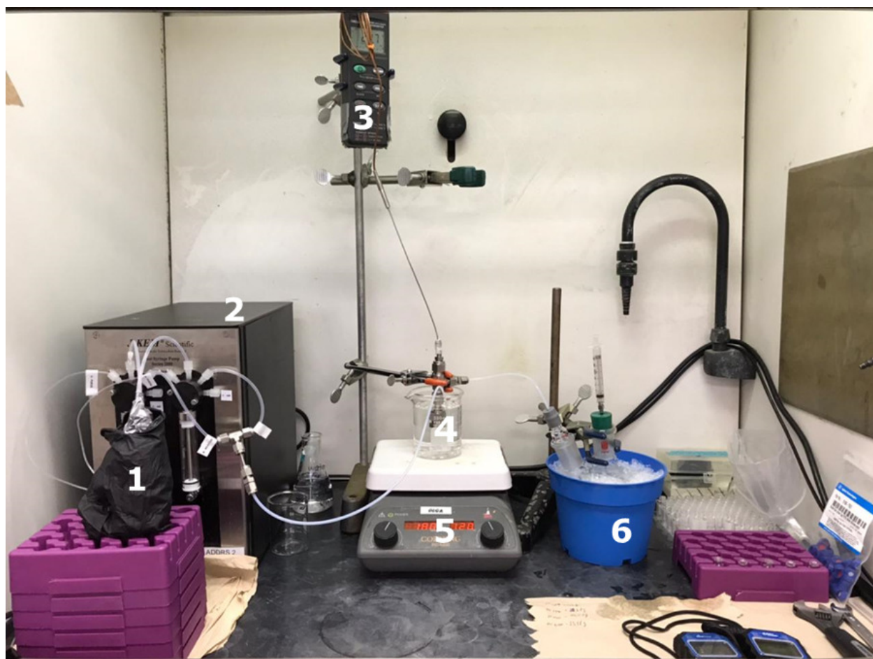
Figure 3.1 Lab-scale setup. 1: TBA+ \text{H}_2\text{O}_2 solution, 2: Pump, 3: thermometer, 4: water bath, 5: heating plate, 6: ice quench.
