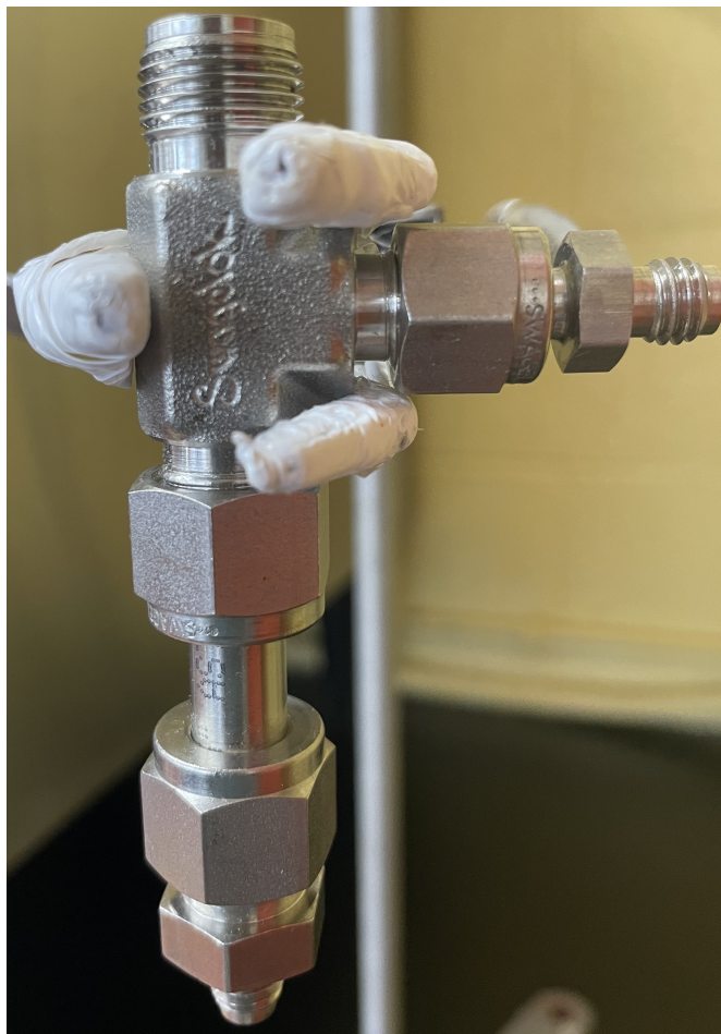
Figure 3.3 Reactor configuration: 3.5 mL plug flow reactor.
