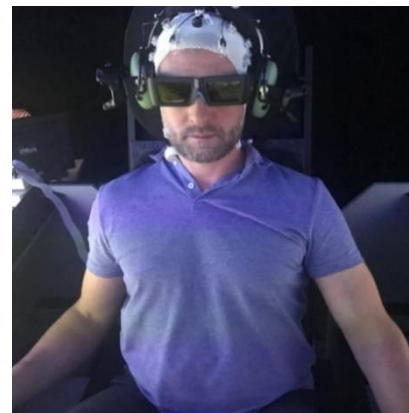
Figure 8.3 - Head tracker and 3D glasses
