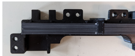
Figure 5.8 Probe pole fabrication with soft steel laminations
