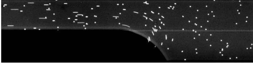
Figure 3.3 Fluorescent microspheres (4.8  $\mu\text{m}$  diameter) revealing stagnancy of the flow far from the receding meniscus. (See Video A.15)
