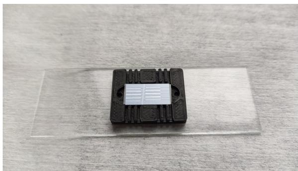
Figure 5.7 Chip placed on the loading pad.
