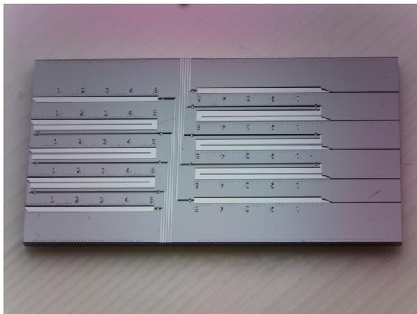
Figure 5.6 Brightfield image of the entire chip with control channels (high inlet hydraulic resistance on the right side).
