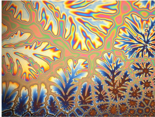
Figure 2.10 Saffman-Taylor viscous fingering resulting from the air displacing a spin coated thin film. The colours are resulting from thin-film interference.<sup>7</sup>
