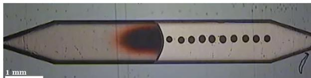
Figure 3.1 Resuspension of printed amaranth dye in a microchannel. Accumulation of dye at the capillary front because of convection and spreading of the concentration profile by TAD.
